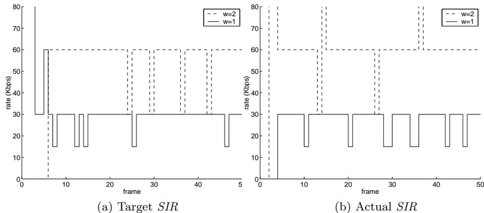
**Fig. 5.** Rate (discrete values) as function of frame number.  $PCE = 0, SIR_{err} = 1$  dB
