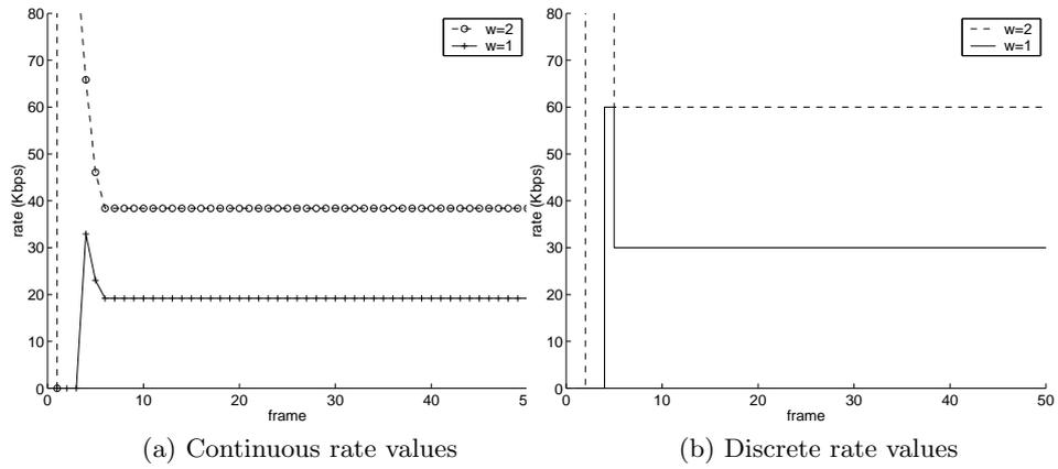
**Fig. 2.** Rate as function of frame number, when rate allocation is based on the target  $SIR$ .  $PCE = 0, SIR_{err} = 0$
