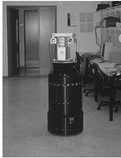
Figure 9: TALOS, the multisensor mobile robot of ICS FORTH.
