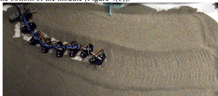
**Figure 5: Polychaete robotic prototype moving on sand**
