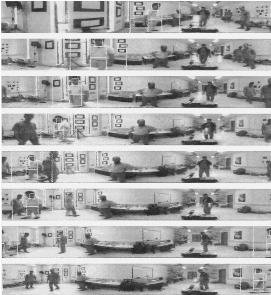
Figure 2. Unfolded panoramic images: person tracking sequence.
