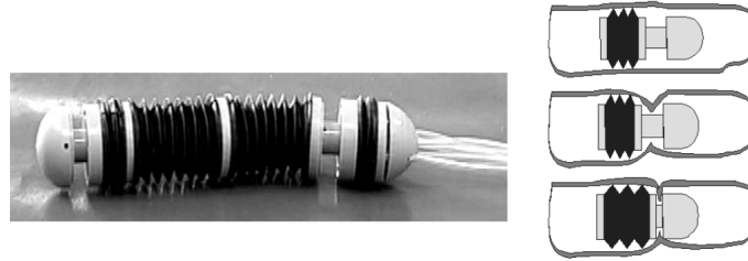
Figure 2. (a) Typical inchworm prototype with ‘suction + clamping’ mechanisms (diameter 24 mm; retracted length 115 mm). (b) Working principle of the clamping mechanism.
