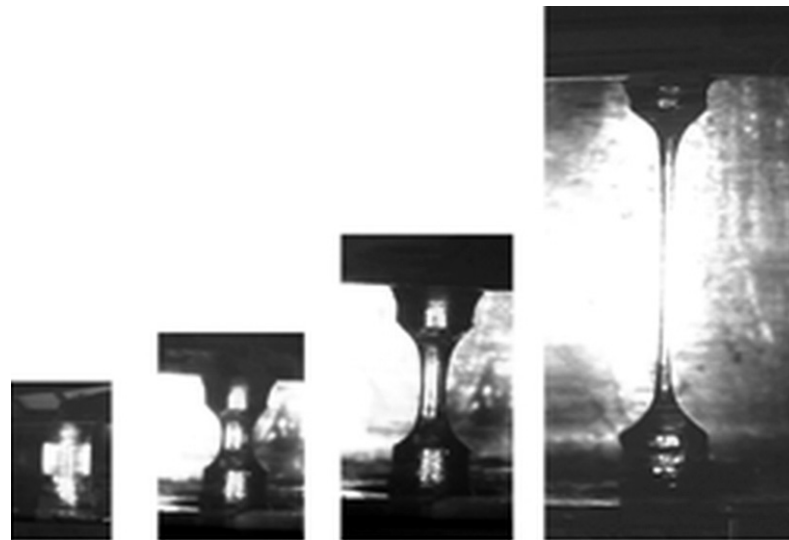
Figure 10. Four phases of the liquid bridge formation.
