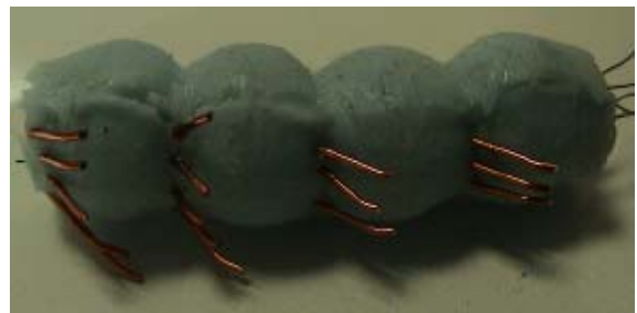
Figure 10. Legged artificial earthworm. The legs, mimicking the setae, are 500 \mu\text{m} in diameter.
